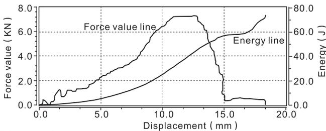
Note: As the chart shows, energy is absorbed by a lower reaction force at the beginning of the stroke, then by a smooth linear deceleration. It decelerates smoothly at last.
